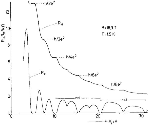
Fig. 2. Gate voltage dependence of the measured Hall resistance  $R_H$  and resistivity  $R_x$  at  $B=18.9\text{ T}$  for a long silicon MOS device (length to width ratio  $L/W=8$ , distance between potential probes  $\Delta=L/3$ ).
