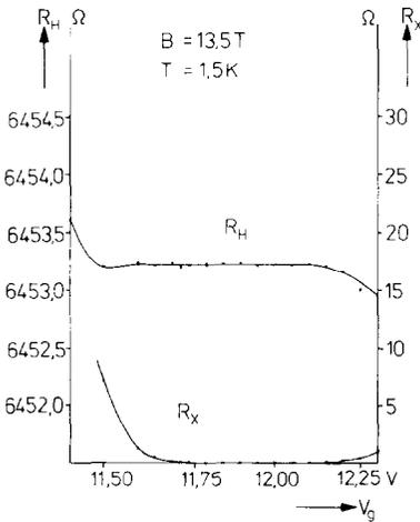
Fig. 3. High-resolution measurements of the Hall resistance  $R_H$  and the resistivity  $R_x$  for a silicon MOSFET at gate voltages close to the occupation of the  $n=0$  Landau levels (after ref. [21]).
