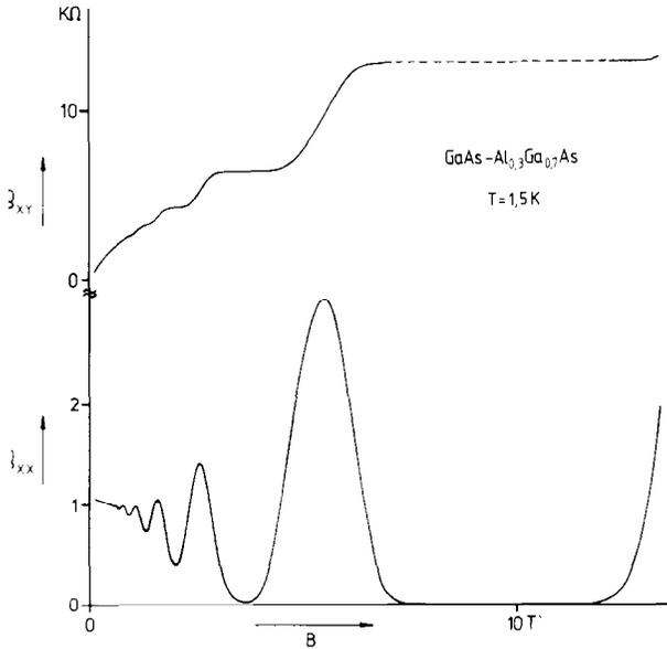
Fig. 4.  $\rho_{xy}$  and  $\rho_{xx}$  measurements on a GaAs-Al<sub>0.3</sub>Ga<sub>0.7</sub>As heterostructure as a function of the transverse magnetic field. The inversion carrier concentration is about  $5 \times 10^{11} \text{ cm}^{-2}$  [21]).
