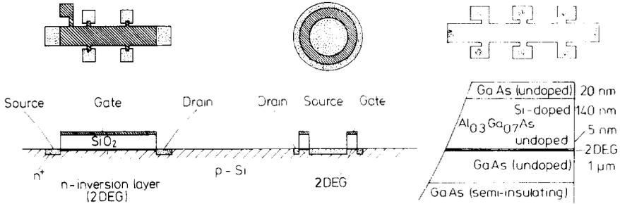
Fig. 1. Typical geometries and cross-sections of devices used in the experiments. From left to right: (a) Long silicon MOS device (Hall geometry) with potential probes (for  $R_x$  measurements) and Hall probes (for  $R_H$  measurements); typical length: 0.5 mm. (b) Circular MOS device for  $\sigma_{xy}$  measurements. (c) Cross-section and top view of a GaAs-Al<sub>0.3</sub>Ga<sub>0.7</sub>As heterostructure with Hall geometry.
