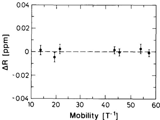
Fig. 2. Differences of the QHR measured in seven GaAs heterostructures. After Ref. [5].
