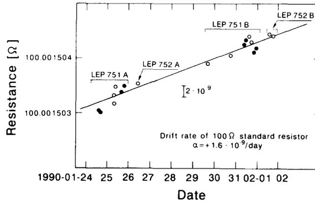
Fig. 1. Comparison of different quantized Hall resistances measured on four GaAs-based heterostructures. The  $100\ \Omega$  standard resistor has an established drift rate of  $1.6 \times 10^{-9}$  per day. After Ref. [4].
