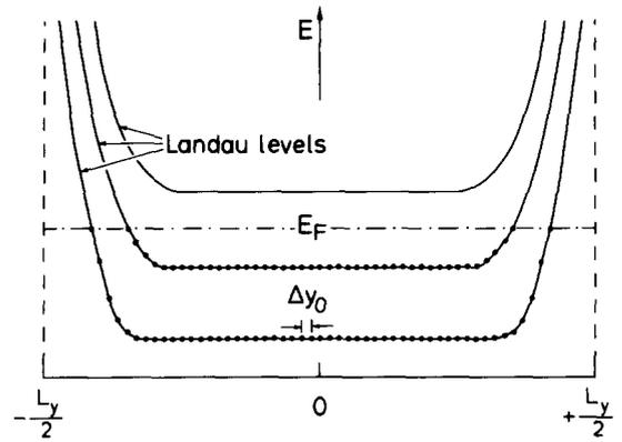
Fig. 5. Energy spectrum of ideal Landau levels for a sample with finite width  $L_y$ .
