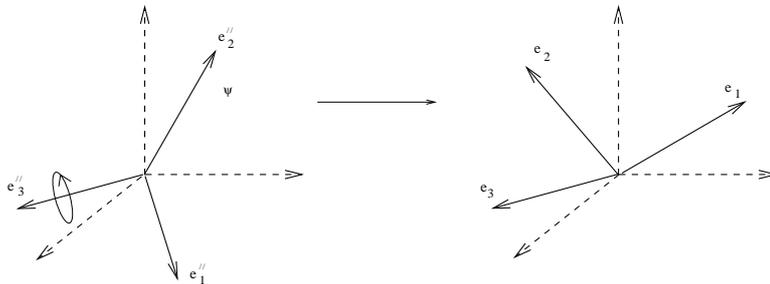
**Figure 39:** Step 3: Rotate around the latest axis  $\mathbf{e}''_3$ .
